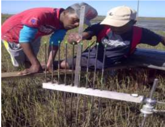
MSc student Athi Mfikili (right) and intern Reanetsi Pohlo measuring sediment elevation with a Rod Set Elevation Table in the Swartkops River estuary
