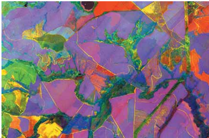
Figure 3.73 An adapted CASI hyperspectral image used for classification of Eucalyptus and Acacia species in KwaZulu-Natal, South Africa. Forests show up in purple and agriculture/fallow land in green hues in this representation.
