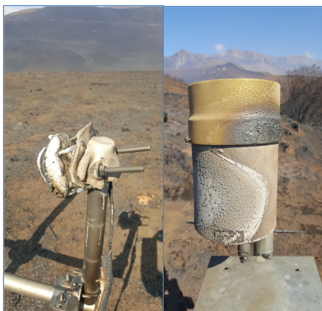
Weather instruments destroyed by a wildfire at Cathedral Peak
