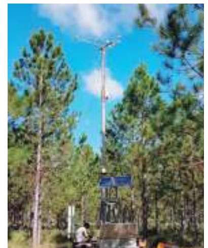
Mobile eddy covariance system measuring pine ET
